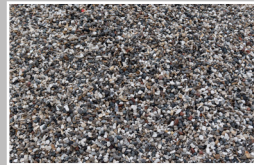
20mm Washed Pipe Bedding
