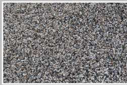
10mm Washed Pipe Bedding
