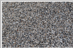
10mm Washed Pipe Bedding
