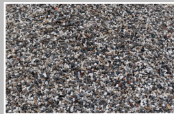
20mm Washed Pipe Bedding
